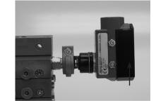
MCSA2503 w/automotive type 3 pin connector Because they use a magnet to sense piston position, entry of contaminants into the system is prevented. These cycle switches may be installed in the end of M2500G valve size '15' and larger. The SPDT switch is rated at 250 VAC/28 VDC-5 Amps. (See Automotive-Type Connectors below)
